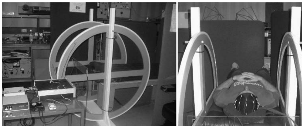
Fig. 1 The design of magnetic field exposure system consisting of Helmholtz coils and a signal generator
